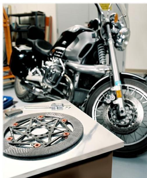
STARBlade® PTCC Motorcyle Brake Rotor
